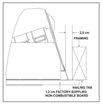
Figure 5.5 Front Side Finishing Detail
